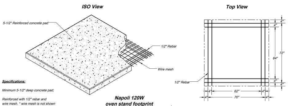
wire mesh. \* wire mesh is not shown in some views for print clarity;
