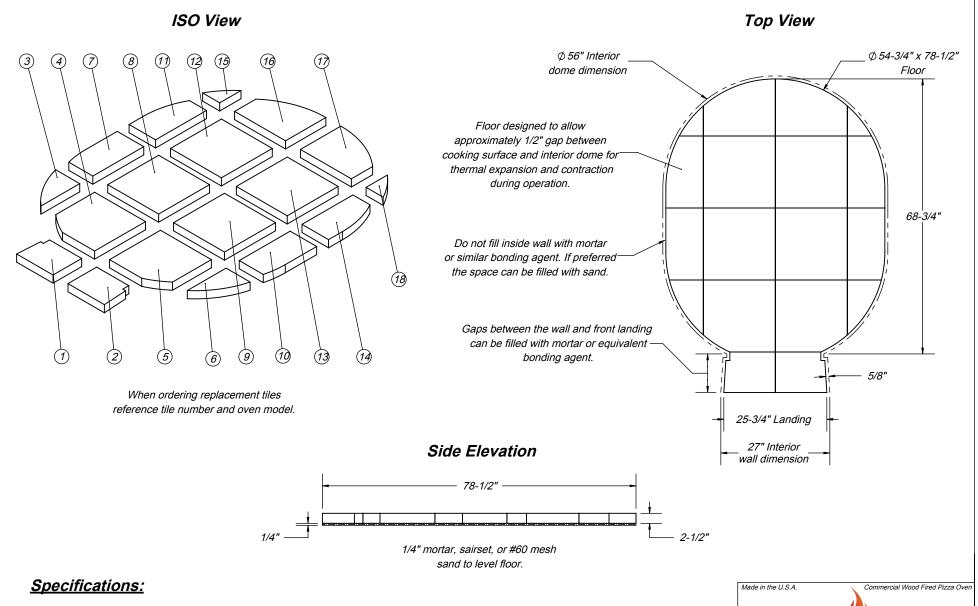
Floor is NSF-4 rated with 2-1/2" thick surface.
