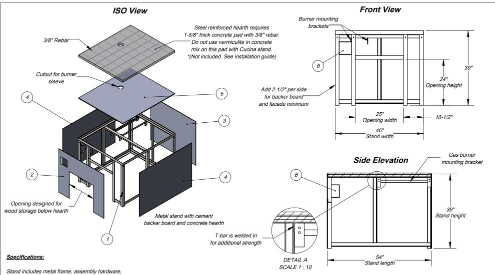
Stand includes metal frame, assembly hardware, precut / predrilled exterior cement backer board panels.
