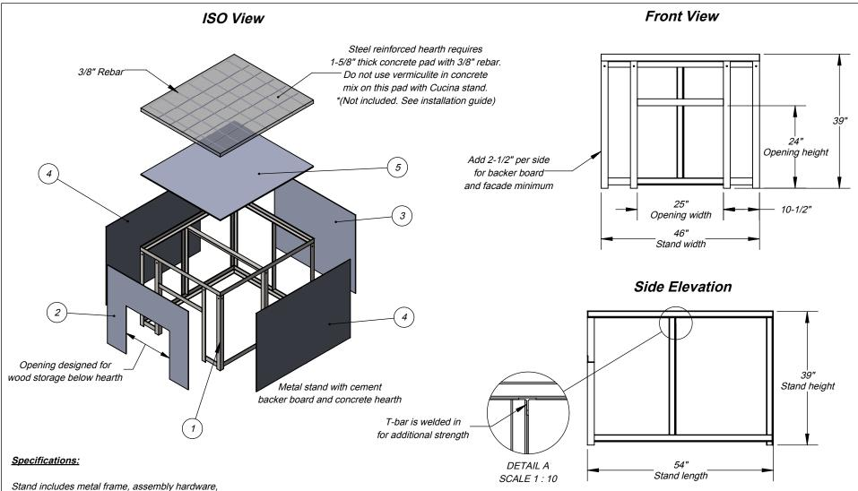
precut / predrilled exterior cement backer board panels.
