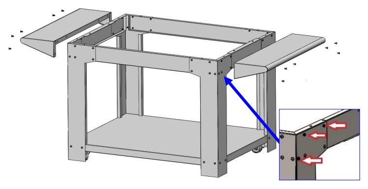
• 1/4" Split Washers (Item #15) and 1/4-20 x1/2" Screws (Item #14) should be inserted into the three pre-drilled holes from the outside of the cart. – Use six washers and six screws per shelf. The correct holes are on the outside edges of the end corners. (See arrows on close-up diagram.)
