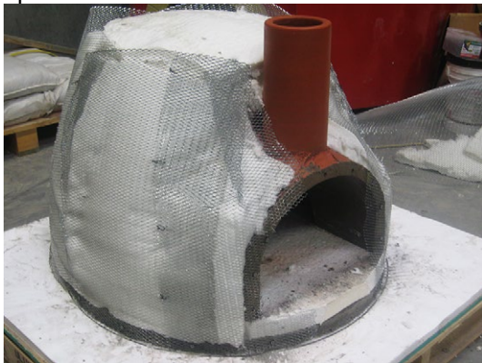
7.1. FB Blanket inside an Igloo frame.
